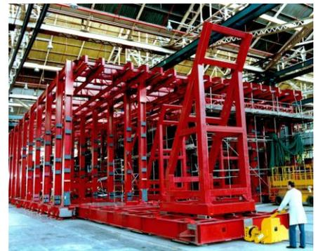
*Airbus A340 wing assembly jigs are moved using air skates and tuggers with a capacity of over 50 tonnes*
